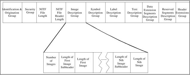
FIGURE 3. <u>NITF file header structure</u>.
